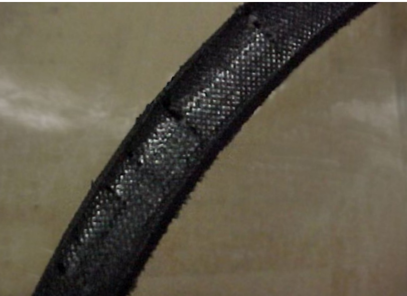
Shiny Side Wall of Un-notched V-Belt
